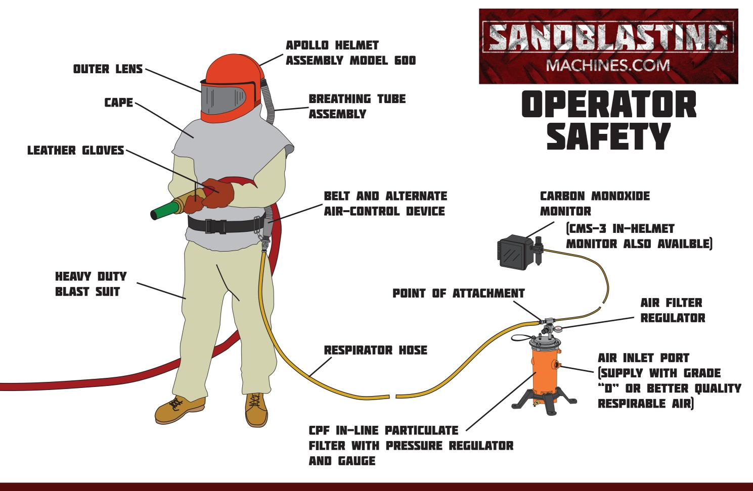
SOME ITEMS ARE POSITIONED FOR CLARITY. THE FILTER AND MONITOR MUST BE PROTECTED FROM THE BLASTING ENVIRONMENT.
