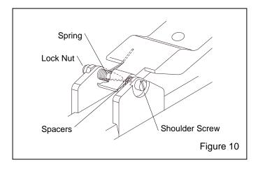
**6.6.3.1** Remove the lock nut from the shoulder screw. Before removing the screw, note the positions of the spacers and spring as shown in Figure 10. The bent end of the spring is against the handle lever, facing up. The straight end is against the body, facing down.
