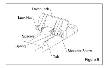
**6.6.2.3** Make sure the lever lock moves freely, raises to full up position, and that the handle lever will not engage unless the lever lock is pulled down.
