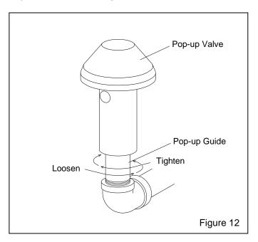
**6.8.3** Using a small pipe wrench, unscrew the pop-up valve guide by turning it counterclockwise. Remove the pop-up valve and guide from the machine.
