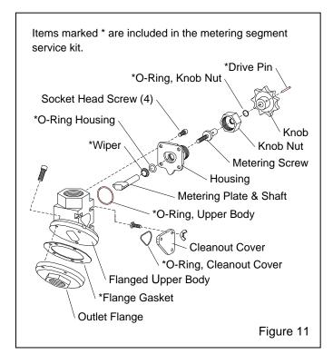
**6.7.11** Remove the o-ring from the knob nut, and remove the o-ring and wiper from the housing.
