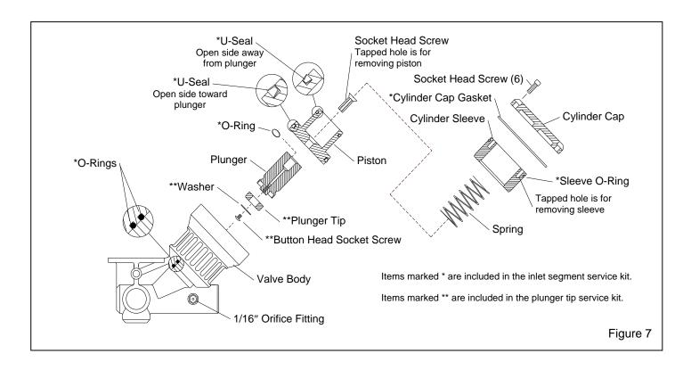
**6.3.9** Replace both o-rings in the valve body.
