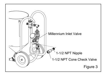
**2.2.2** Use a Clemco 1-1/2-NPT cone check valve, Stock No. 02296. A smaller size valve could restrict air movement and reduce nozzle pressure. Do not use a swing check valve, as the swing gate may break in blast machine applications. When installing the valve, make sure the directional arrow is pointing with the air flow, toward the machine.
