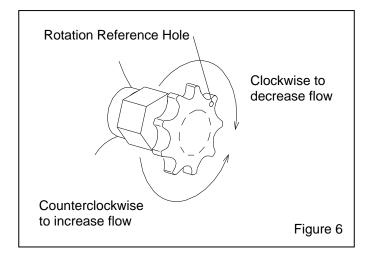
**4.1.4** Optimum abrasive flow depends on the type and size of abrasive and blasting pressure, and can best be determined by experience. Use as little abrasive as possible while maintaining the maximum cleaning rate. The air/abrasive mixture should be mainly air. As a rule, the stream of abrasive coming out of the nozzle should barely discolor the air when seen against a contrasting background.
