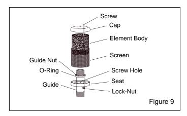
**5.10.5** Make sure the guide nut is fastened tightly to the guide.
