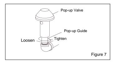
**5.8.5** Slide the new pop-up valve over the guide, and then screw the valve guide (with the pop-up valve on it) into position inside the machine. Tighten the guide snug, but not wrench-tight. Over-tightening the guide will make it difficult to remove the next time the pop-up valve needs replacement.
