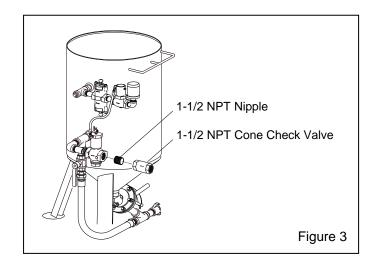
**2.3.2** Use a Clemco 1-1/2-NPT cone check valve, Stock No. 02296 or equal purchased from a local source. A smaller size valve could restrict air movement and reduce nozzle pressure. Do not use a swing check valve, as the swing gate tends to break in blast machine
