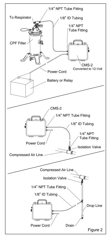
**2.1.2.5** The tee in the air supply line should face up to prevent water from accumulating in the sample—air line. If the tap cannot face upward, install a drop pipe and drain to prevent water from entering the monitor.
