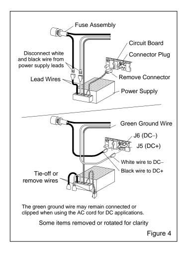
**2.5.10** Attach a positive (+) terminal connector to the end of the black wire and a negative (-) connector to the end of the white wire. Clip the green wire.
