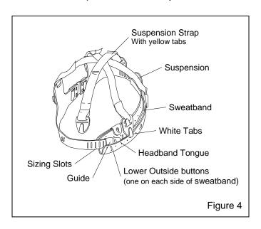
**6.1.3** The suspension fits head sizes 6.5 to 8. Head sizes are marked on the headband slots. Slide the headband tongue in or out of the guide to attain the
