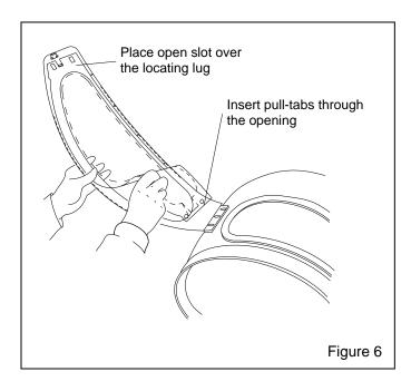
**9.1.1.9** Snipping off the pull-tab on the innermost lens after the frame is closed will prevent unintentional removal of the last lens and prolong the life of the inner lens.
