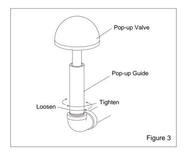
**5.3.5** Slide the new pop-up valve into the guide, and then screw the valve guide (with the pop-up valve in it) into position inside the machine. Tighten the guide until wrench-snug, but not wrench-tight. Over-tightening the guide will make it difficult to remove the next time the pop-up valve needs replacement.
